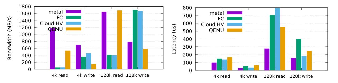
Hardware supports 340,000 IOPS; 1 GB/s at 4k; serial access to disk harms FC performance
